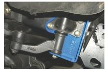
Our simple bolt-on idler arm brace creates a double shear mounting point for the factory idler arm spindle shaft. It eliminates the side loading force generated by big tires bouncing off of big rocks! Cheap insurance against snapping the entire assembly off and becoming stranded. Laser crafted for perfect fit. Finished in CALMINI bright blue powder coat. Fits 98-03 Xterra/Frontier Part # NP12490 \$34.95
