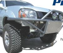
CALMINI Prerunner Bumpers are a fully bolt-on replacement unit for your stock front bumper. Constructed from 2" x .120" wall tubing for maximum strength it mounts directly to the stock frame rails, 3/16" 6061 aluminum skid plate is included standard.
