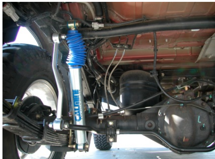
Overall rear installation: brake lines, spacer, shocks, sway bar links, leaf springs, and u-bolts.
