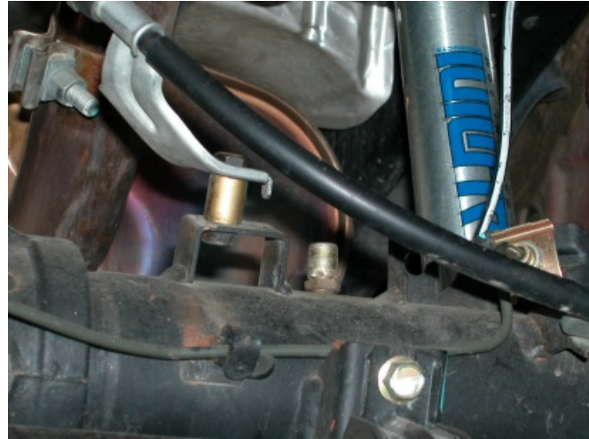
Hard brake line spacer installed on passenger side of rear axle housing.
