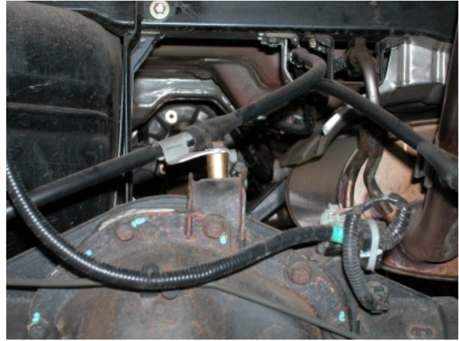
Hard brake line spacer installed on top of rear differential.
