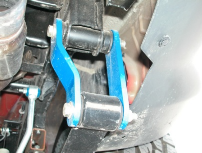
Rear spring shackle correctly installed on the rear replacement leaf spring using supplied hardware and sleeves.
