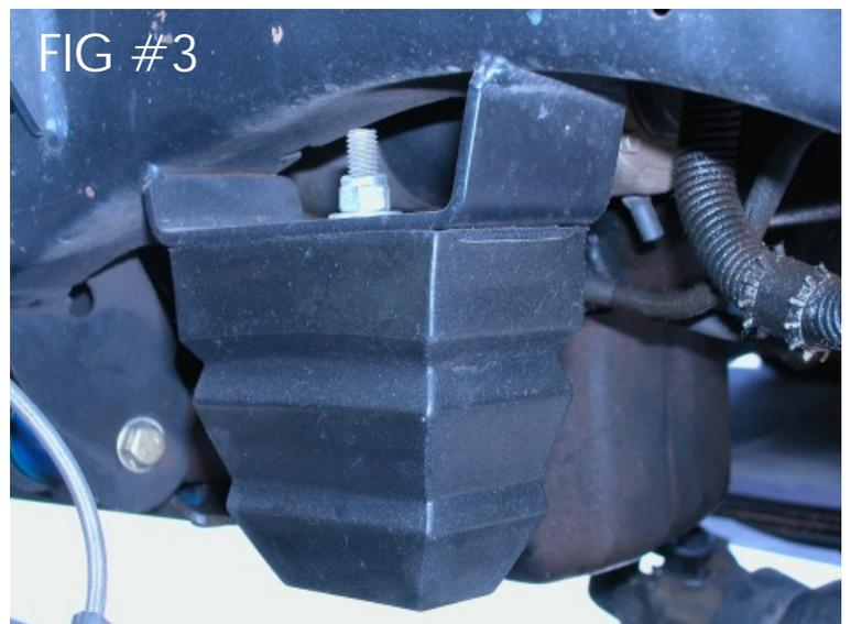
3. Once the perch and bump stop plate have been tacked into place and the suspension has been cycled with all parts snugly installed, the spring and strike plate can be removed to allow for complete welding of the parts to the axle and frame. Take caution to watch for warpage or movement of the parts when welding.
